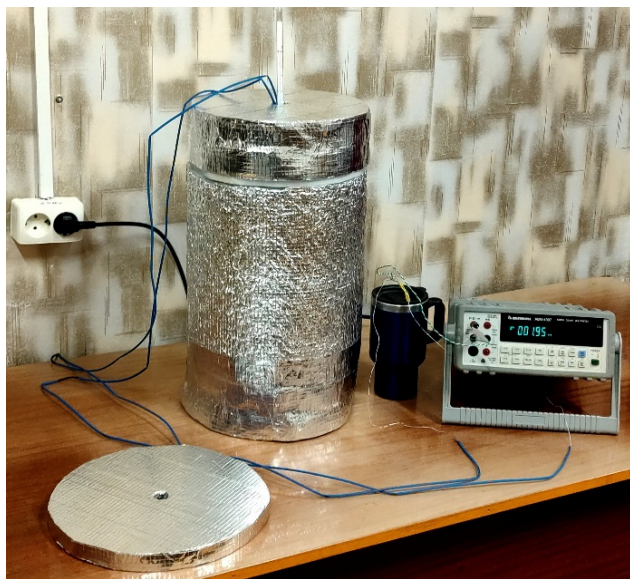
Figure 2. Experimental unit for thermocouple calibration with expedient insulation radius [46]
