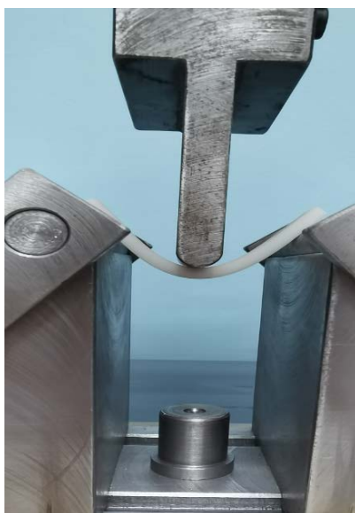
Figure 3. Three-point bending testing of the specimen.
