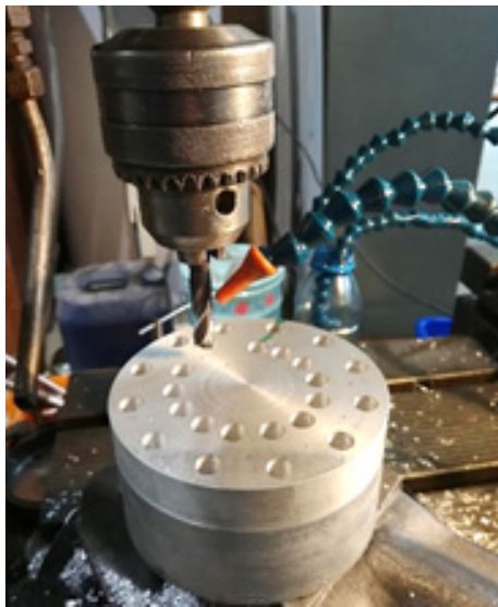
Figure 2. Composite drilling station with external oil mist supply
