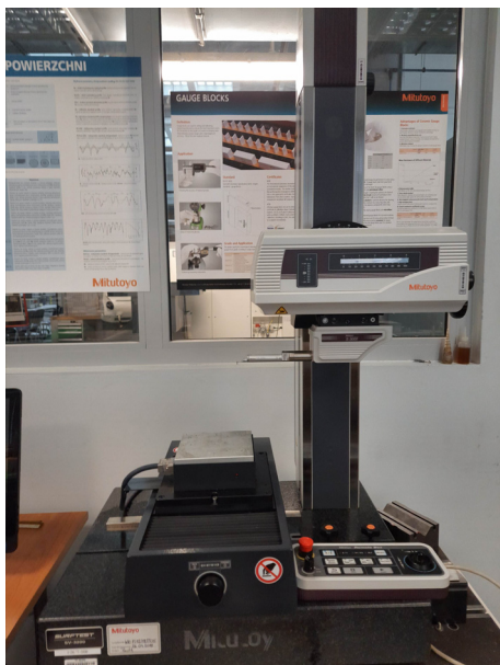
Figure 3. SURFTEST SV – 3200 device for measuring surface roughness
